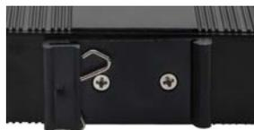
To install the wall mount, the DIN-Rail kit must be replaced by the mounting bracket
