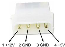
To use the PoE function of the EX-6072PoE-2 and to supply the end devices with power, the card must be connected to the power connector of the PC power supply! Only one power connector may be used J3 OR J4!
